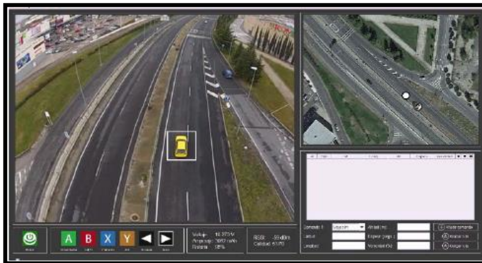
Figure 2.9: Screenshot of the developed software during a flight where the yellow car (in the frame) is the objective to track.
