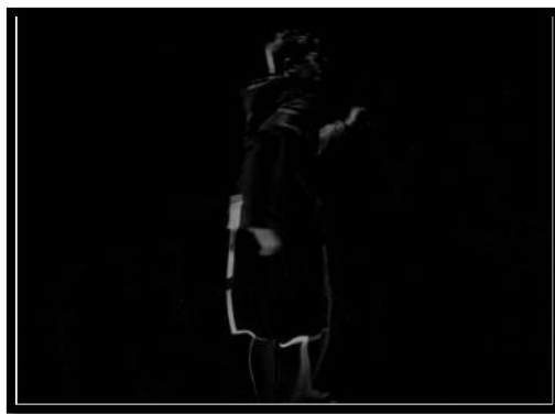
Figure 2.2: Image after the subtraction of subsequent frames.
