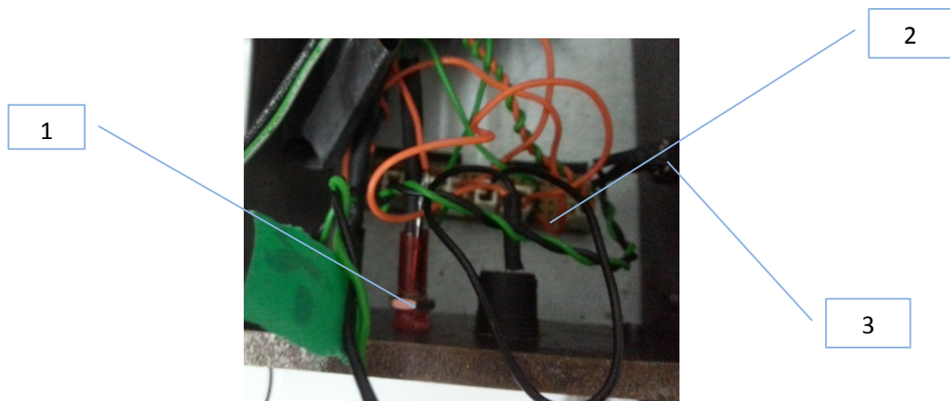
Figure 4.3: Led and Switch
