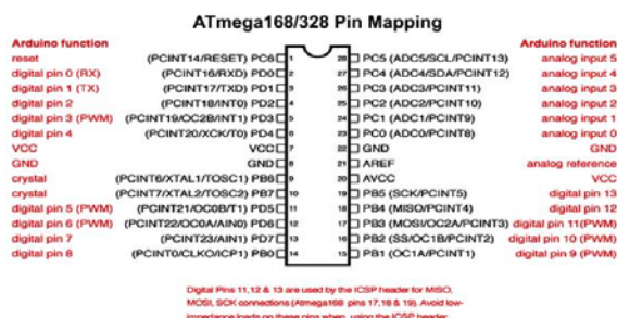
Figure 2.9: Pin diagram of Atmel ATmega328
