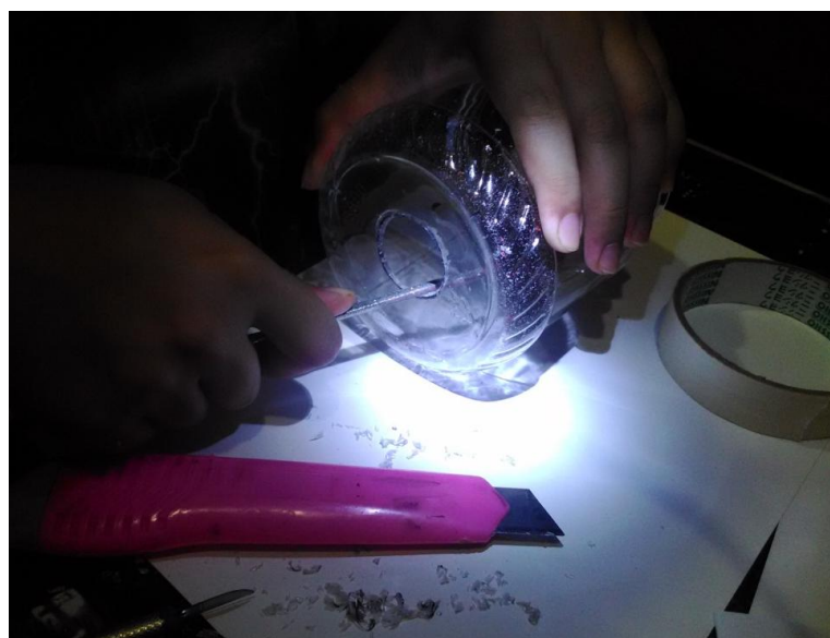
Figure 3.13: Filing the fish feeder body.
