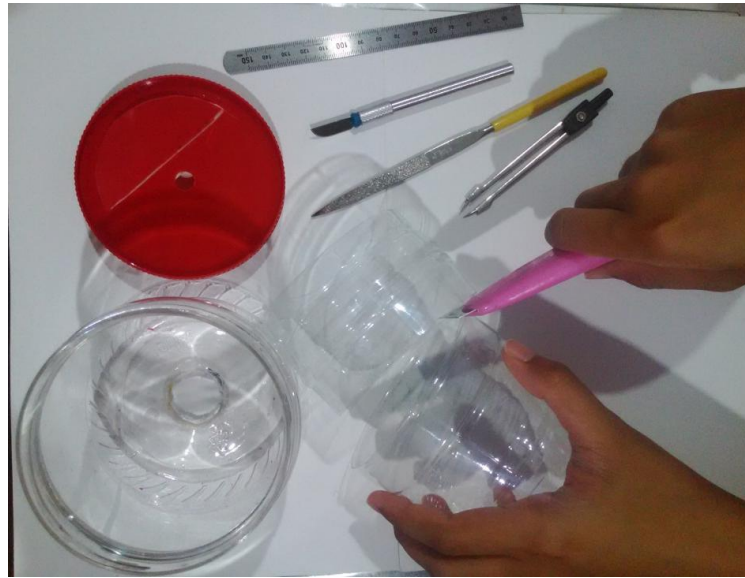
Figure 3.12: Cutting the fish food container.
