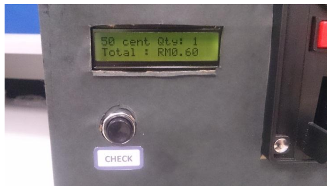
Figure 4.9: LCD display after one 50 cent is inserted
