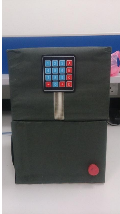
Figure 4.3: The backside of the prototype consists of keypad and security door
