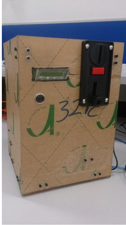
Figure 4.1: The frame of the coin counting and sorting machine prototype
