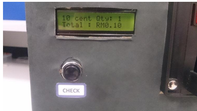
Figure 4.8: LCD display after one 10 cent is inserted
