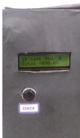
Figure 4.6: Display of 20 cent quantity and total amount of coin
