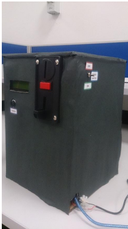
Figure 4.2: The frame of prototype covered with black sugar paper
