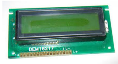
Figure 3.10: LCD with 2 X 16 display
