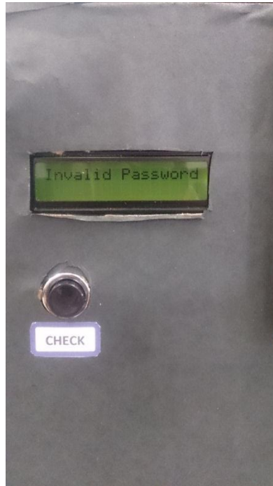
Figure 4.19: Security door cannot open with invalid password
