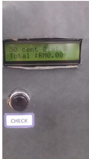
Figure 4.7: Display of 50 cent quantity and total amount of coin
