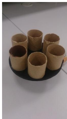
Figure 4.14: Rotary disc with 6 coin slot
