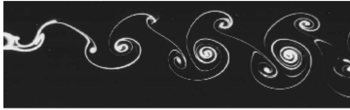
Figure 2.8: Von Kármán Vortex Street, wake pattern behind an oscillating cylinder at Re = 140
