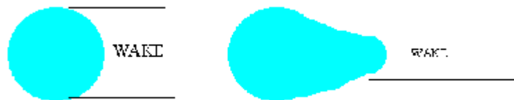
Figure 2.1: Wake occur at the back of bluff bodies
