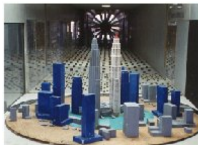
Figure 2.3: PETRONAS Twin Tower model in wind tunnel testing
