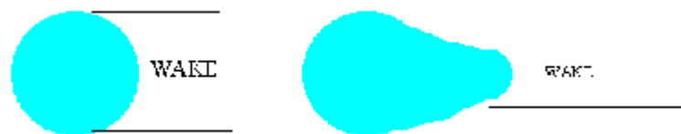
Figure 2.1: Wake occur at the back of bluff bodies
