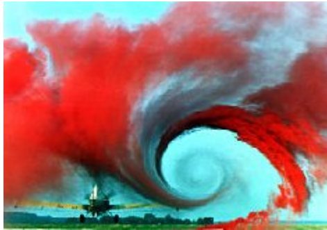
Figure 2.4: Vortex created by the passage of an aircraft wing, revealed by colored smoke
