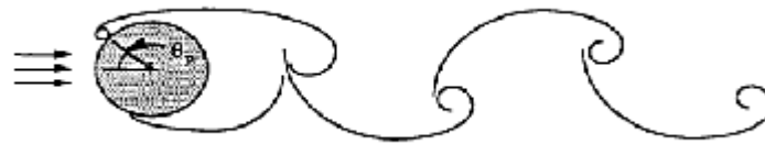
Figure 2.2: Schematic of the bluff body (Circular Cylinder) in 2-Dimensional
