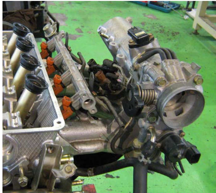
Figure 2.1: Typical intake manifold
