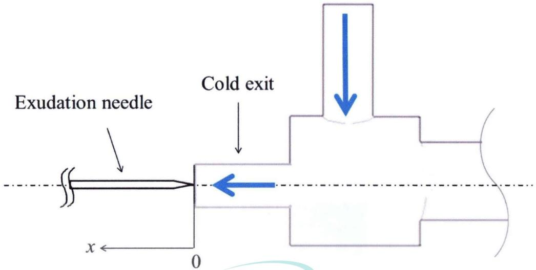
Fig. 4.3 Set up of exudation needle in cold flow
