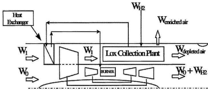
Fig. 1.3 Integrated liquid-O<sub>2</sub> collector plant architecture [4]
