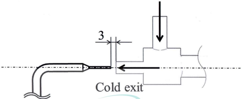
Fig. 4.1 Setup of Pitot pressure probe
