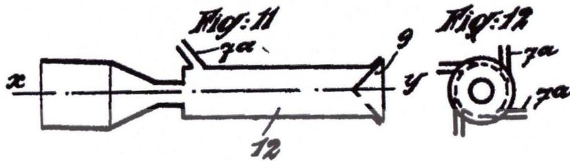
Fig. 1.1 Vortex tube invented by George Ranque [18]
