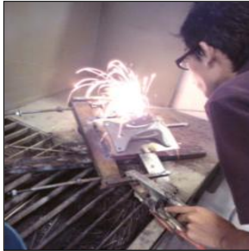
Figure 3.15: Used the Arc welding to make joining
