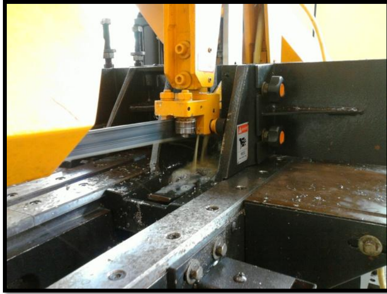
Figure 3.11: Cutting with horizontal bend saw
