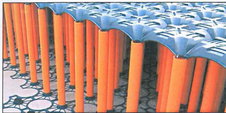
Figure 2.8: Modular slab formwork
