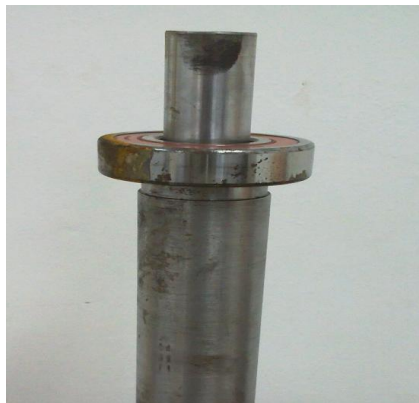
Figure 3.33: The bearing fits perfectly into the shaft after it's diameter has been reduced using turning-lathe process.
