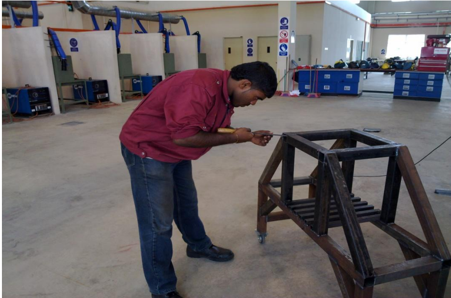
Figure 3.27: Filing is done to remove the sharp edges to make the test rig convenient to the user.
