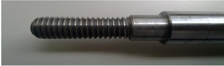
Figure 3.32: The 24mm nut could perfectly slide into the threading
