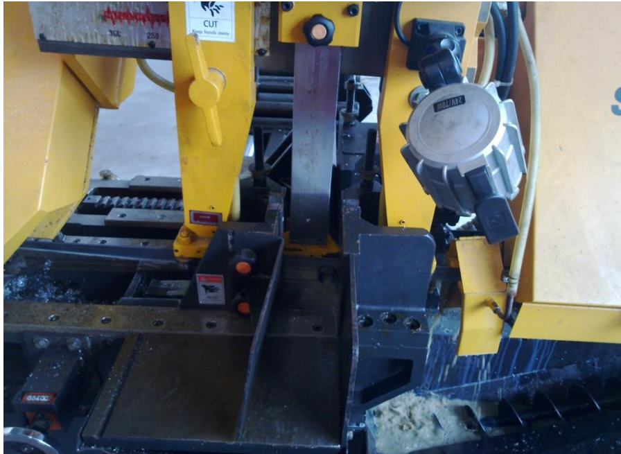
Figure 3.21: Cutting the mild steel rod using bend saw machine.
