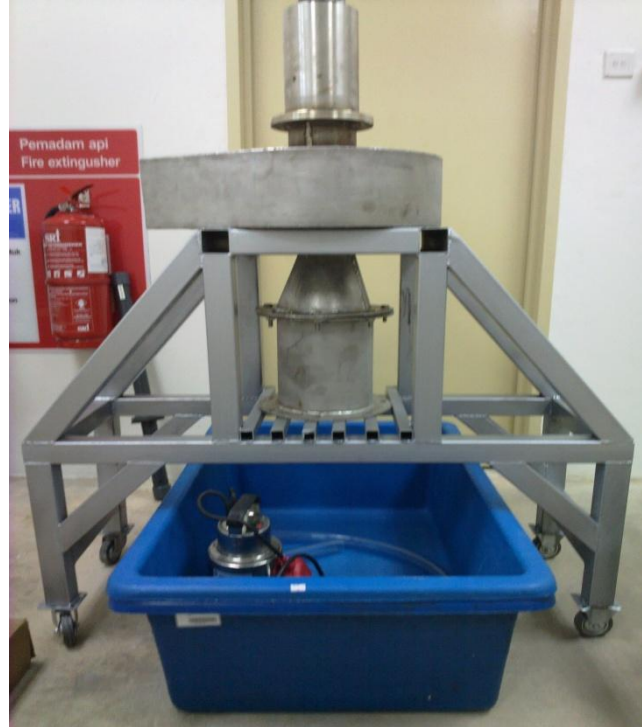
Figure 4.3: Turbine is placed on top of the test rig.
