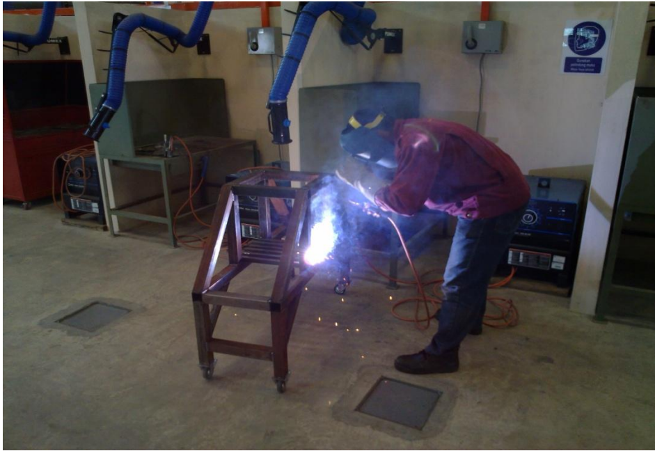
Figure 3.22: Welding the stand using arc welding
