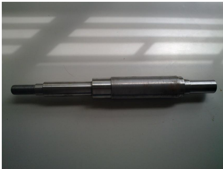
Figure 3.25: This shows the reduced diameter of the shaft and its threading
