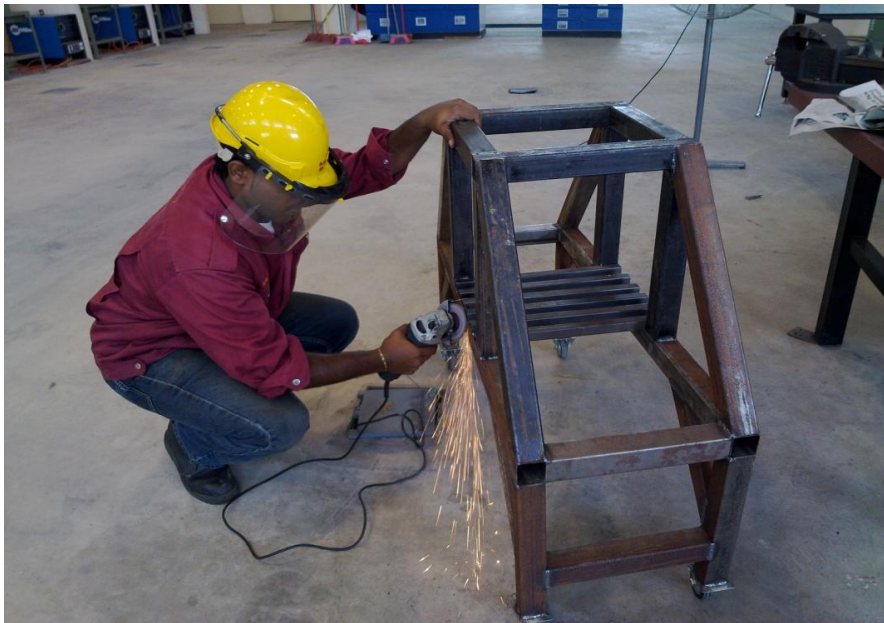
Figure 3.26: Grinding is being done to flatten the extra bits of welding.
