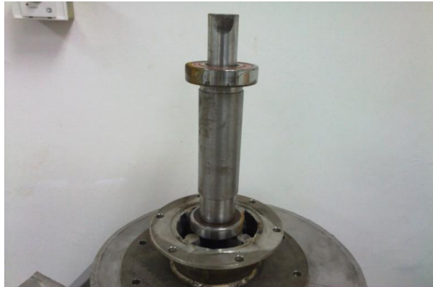
Figure 3.34: The shaft-bearing fits perfectly into the turbine runner cover. The bearing was held stiffly and this avoids the shaft from vibrating while rotating.
