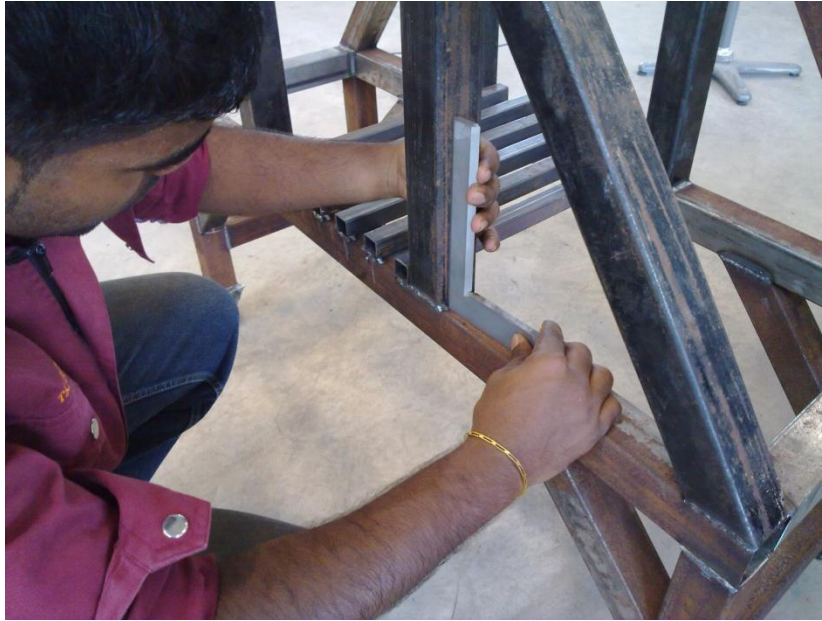
Measure the perpendicularity using l-square
