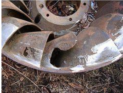
Figure 2.5: Rusted turbine blade
