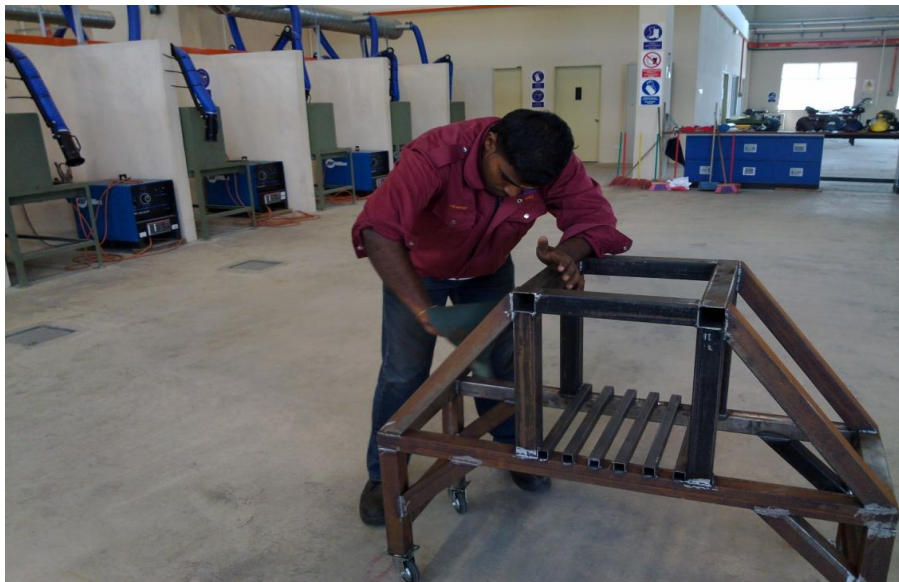
Figure 3.28: Rust is being removed using sand paper to ensure a better surface appearance is achieved.
