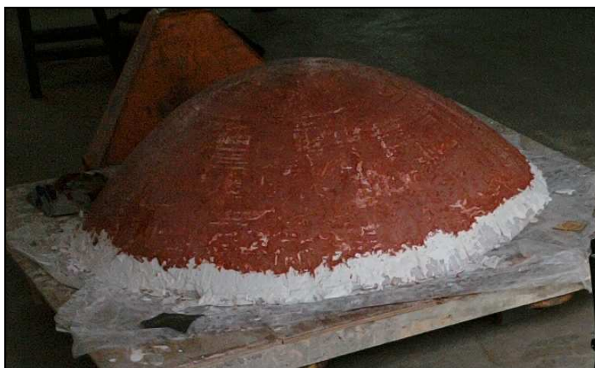
Figure 3.15: Mould ready for glass fibre process
