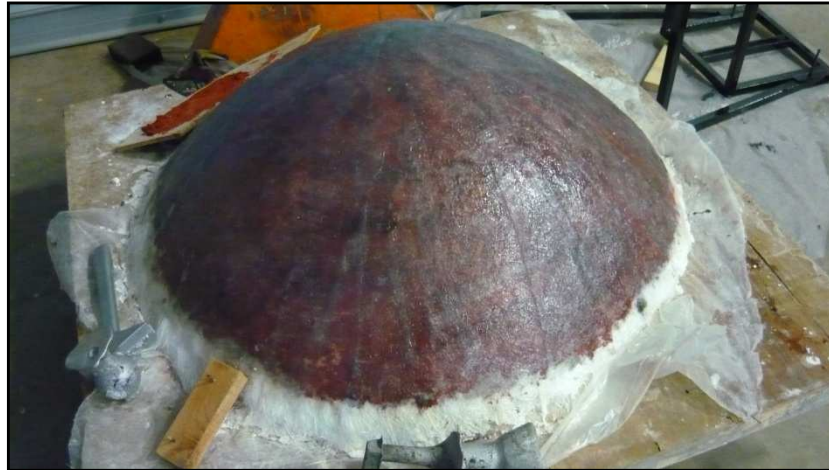
Figure 3.16: Fibreglass process completed
