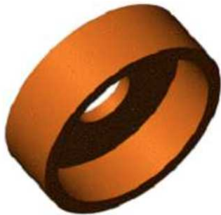
Figure 1. Topology optimized cap-shaped coil [9]
