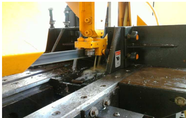
Figure 3.13: Cutting of mild steel bar with bend saw
