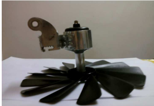
Figure 4.2: Dynamo attached to fan blade
