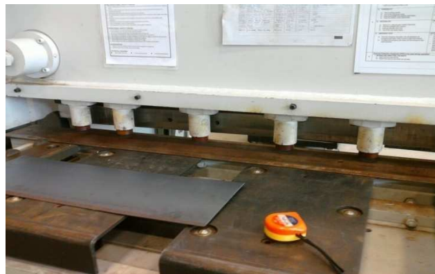
Figure 3.12: Cutting of aluminium alloy plate with pneumatic shearing machine
