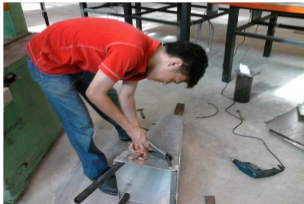
Figure 3.16: Using riveter to rivet the solar tower
