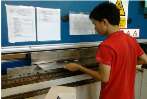
Figure 3.14: Using pneumatic bending machine to bend solar tower
