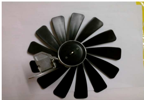
Figure 4.1: Dynamo attached with fan blade
