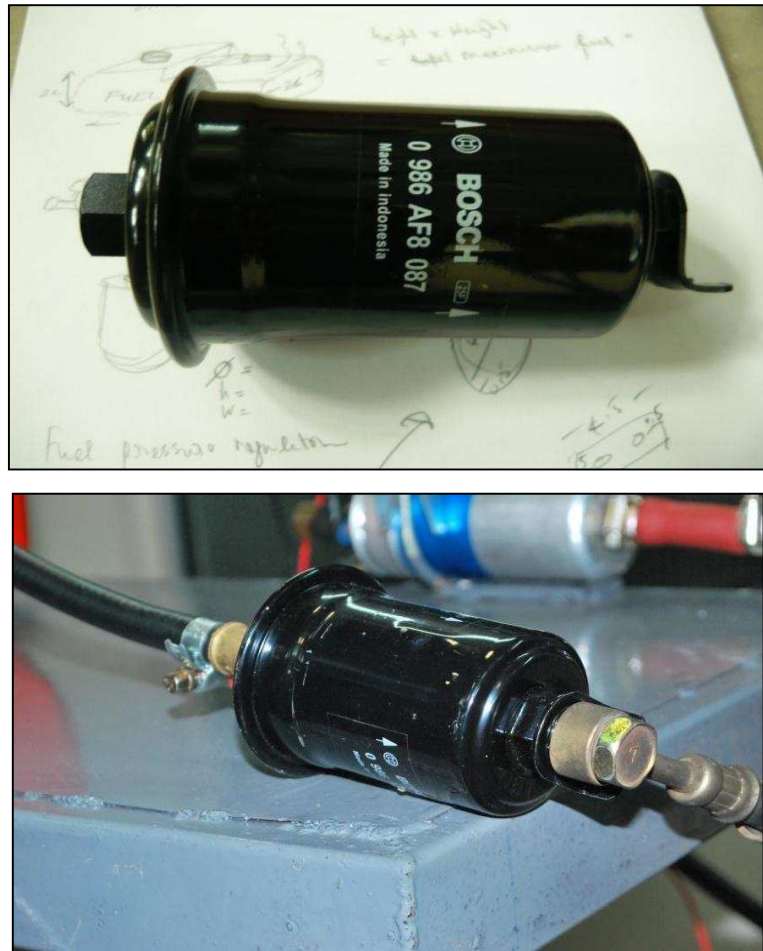
Figure 2.5 Shown a fuel filter that being used on the rig
