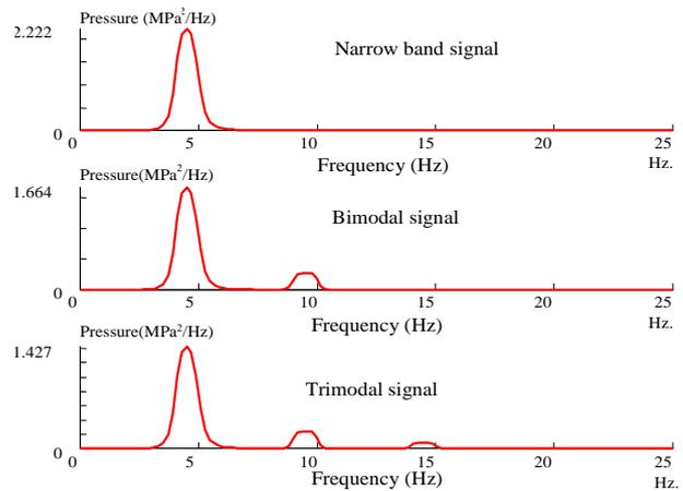
Figure 7. Power spectral density functions of narrow band, bimodal and trimodal signals.
