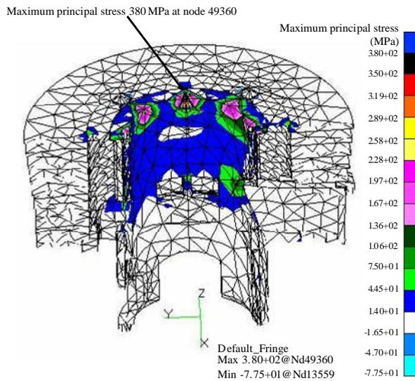
Figure 2. Maximum principal stresses distribution for Pseudo-static linear analysis.
