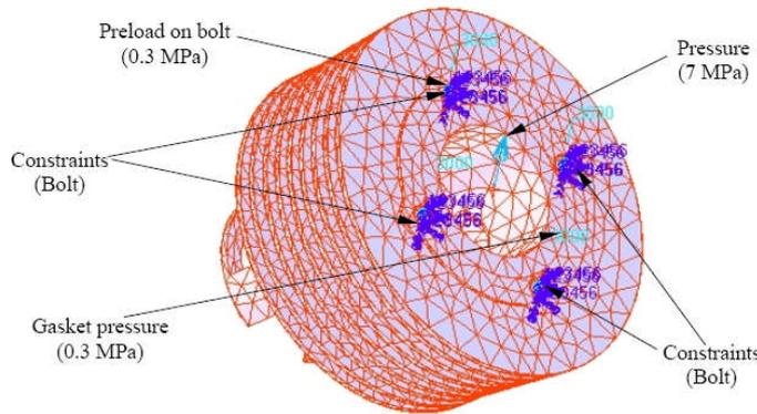
Figure 1. Loading and constraints on the cylinder block.
