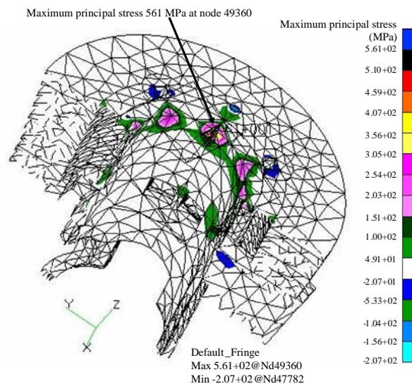
Figure 5. Maximum principal stresses contour for the frequency response analysis with 32 Hz.
