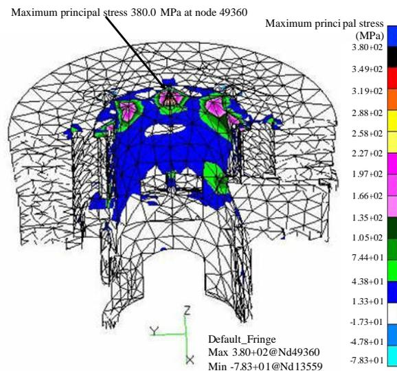
Figure 3. Maximum principal stresses distribution for frequency response analysis with zero Hz.
