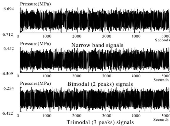
Figure 6. Time-loading histories of narrow band, bimodal and trimodal signals.
