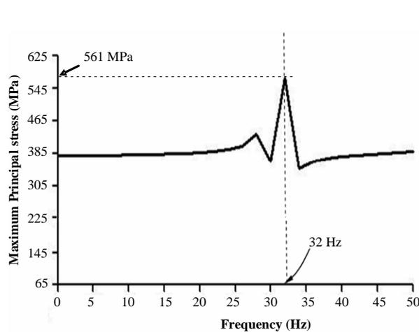
Figure 4. Maximum principal stresses plotted against frequency.
