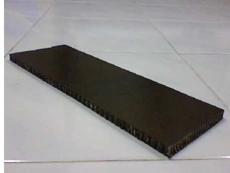
Figure 3.2: Carbon fiber reinforced plastic (CFRP)
