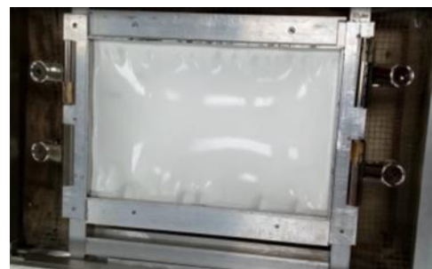
Figure 11. The plastic sheet at sag point
