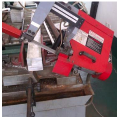
Figure 1. The band saw cutting the aluminum block.
