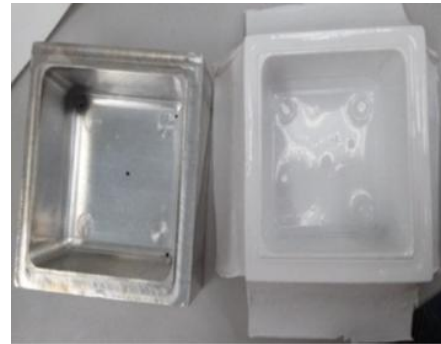
Figure 13. The excess plastic trimmed off
