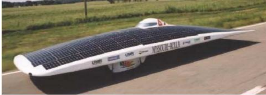
Missouri-Rolla Solar Car, 2003 American Challenge Champion Small Cross-Sectional Area Slightly Curved Underbelly
