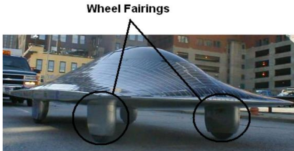
Kansas State Solar Car: Use of fairing on all four wheels
