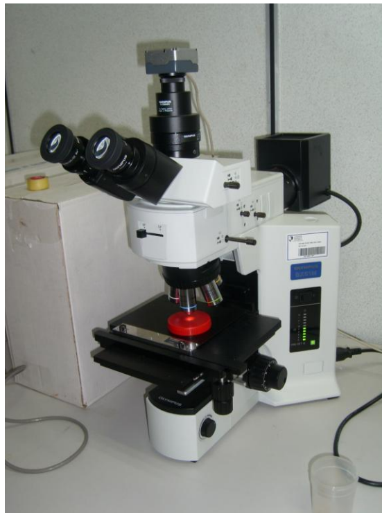
Figure 3.6: OLYMPUS BX51M upright optical microscope
