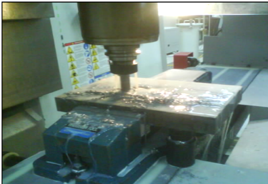
Figure 3.9: Machining process for riser design
