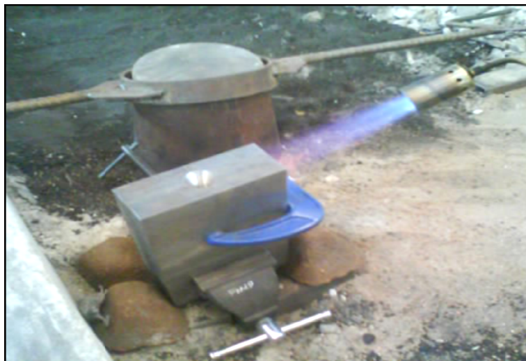
Figure 3.13: Pre-heated the mold
