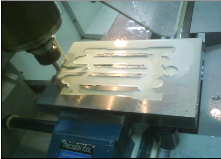
Figure 3.10: Machining process for tapered sprue
