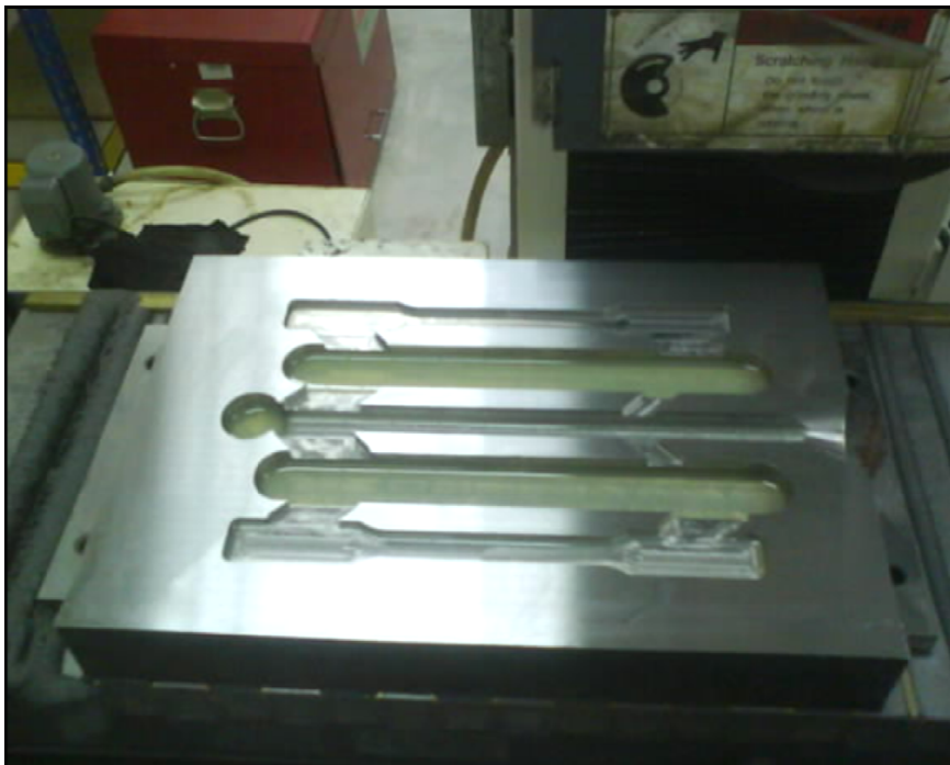
Figure 3.11: Finishing process using surface grinder machine.
