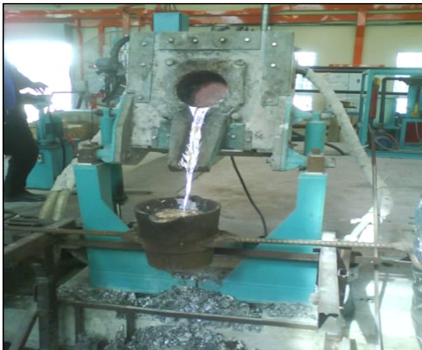
Figure 3.15: Molten metal were carried out from the furnace
