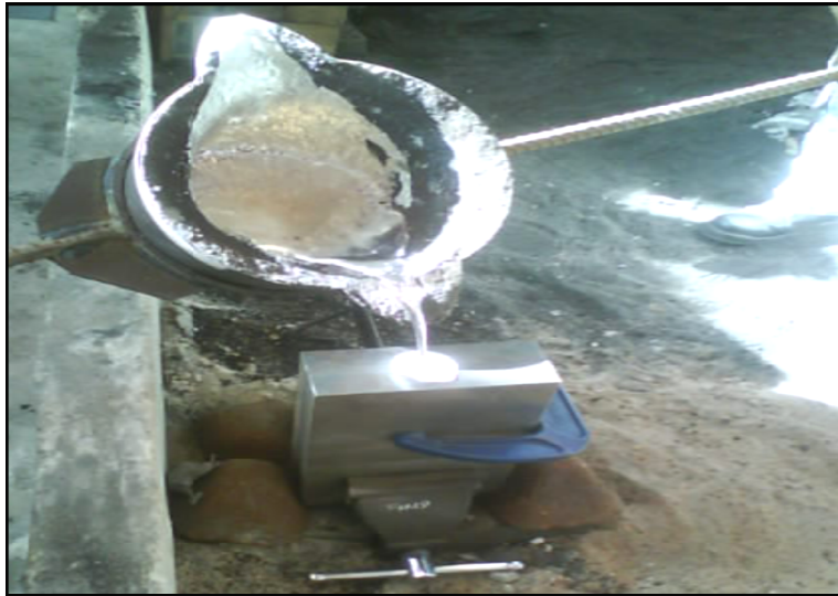
Figure 3.14: Molten metal is poured into the mold
