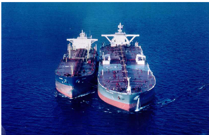
Figure 1.2 : Ships lightering operation [126].
