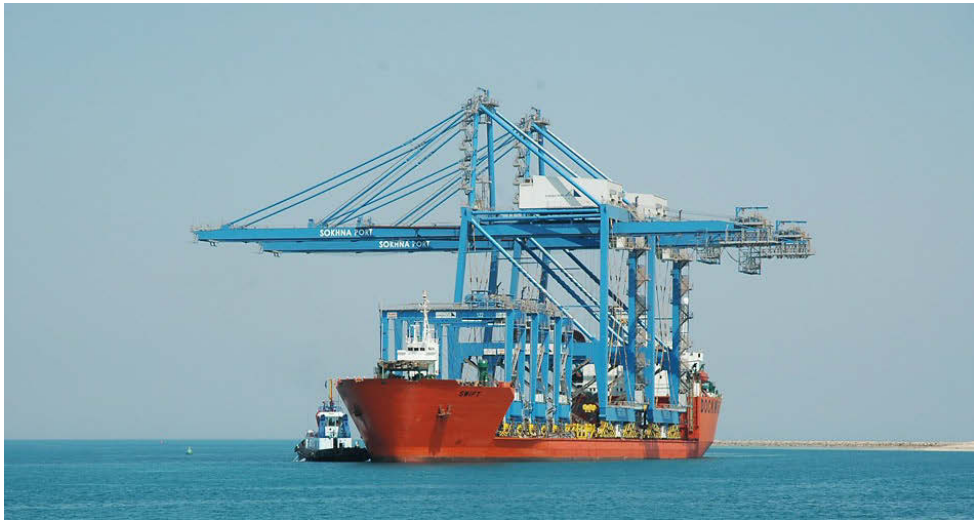
Figure 1.4 : Container gantry crane mounted on a vessel [113].
