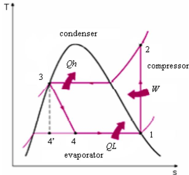
Figure 2.1:  $T$ - $s$  diagram for the ideal vapor compression cycle [8]
