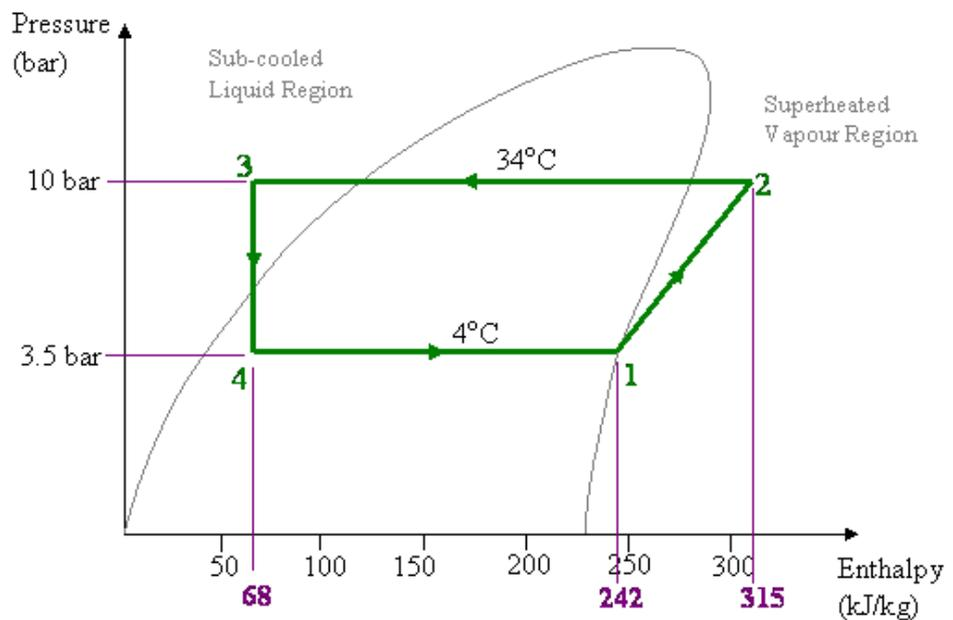
Figure 2.2:  $P$ - $h$  diagram of Refrigeration Cycle for R-134a
