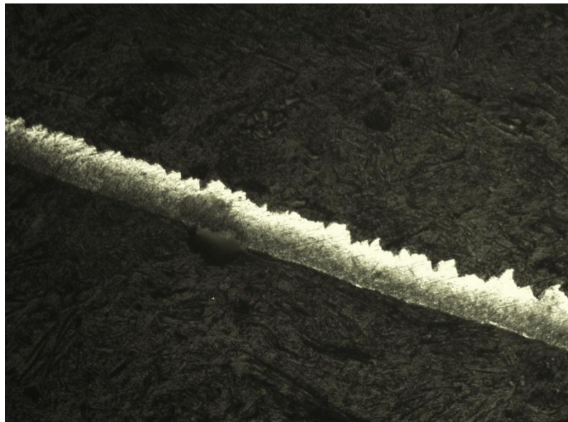
Figure C2.2: Chip structure produced with V= 90 m/min and f= 0.15 mm/rev
