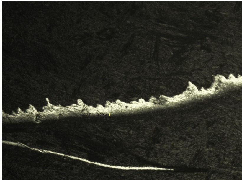
Figure C2.4: Chip structure produced with V= 150 m/min and f= 0.15 mm/rev
