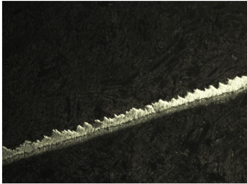
Figure C1.3: Chip structure produced with V = 150 m/min and f = 0.05 mm/rev
