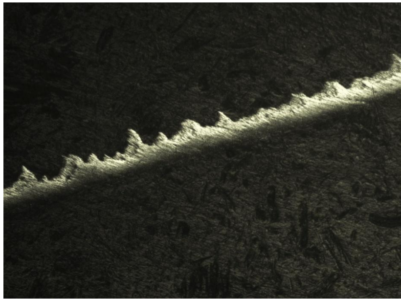
Figure C1.4: Chip structure produced with V = 150 m/min and f = 0.15 mm/rev
