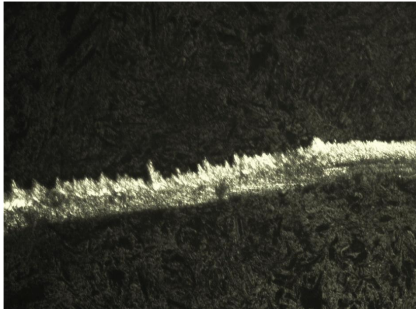
Figure C1.7: Chip structure produced with V= 120 m/min and f= 0.0293 mm/rev
