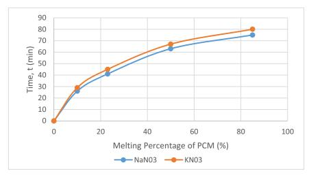
Fig. 6. Time verses PCM Melting rate for both NaNO<sub>3</sub> and KNO<sub>3</sub>.
