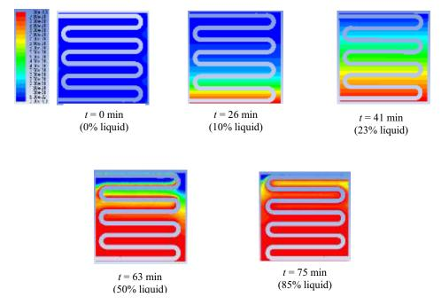
Fig. 5. Liquid fraction of PCM melting phase distribution.
