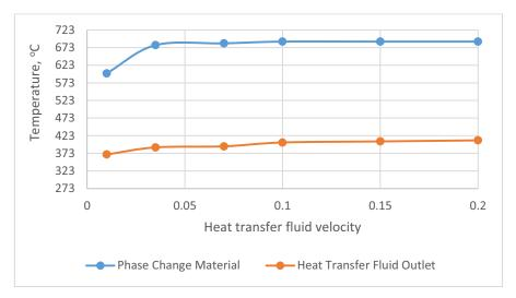
**Fig. 3.** Effect of heat transfer fluid velocity on the temperatures of the phase change material and the HTF outlet.
