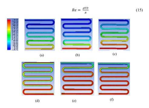
Fig. 2. Temperature distribution in K for different heat transfer fluid velocities (a) 0.01 m/s; (b) 0.035 m/s; (c) 0.07 m/s; (d) 0.1 m/s; (e) 0.15 m/s; (f) 0.2 m/s.
