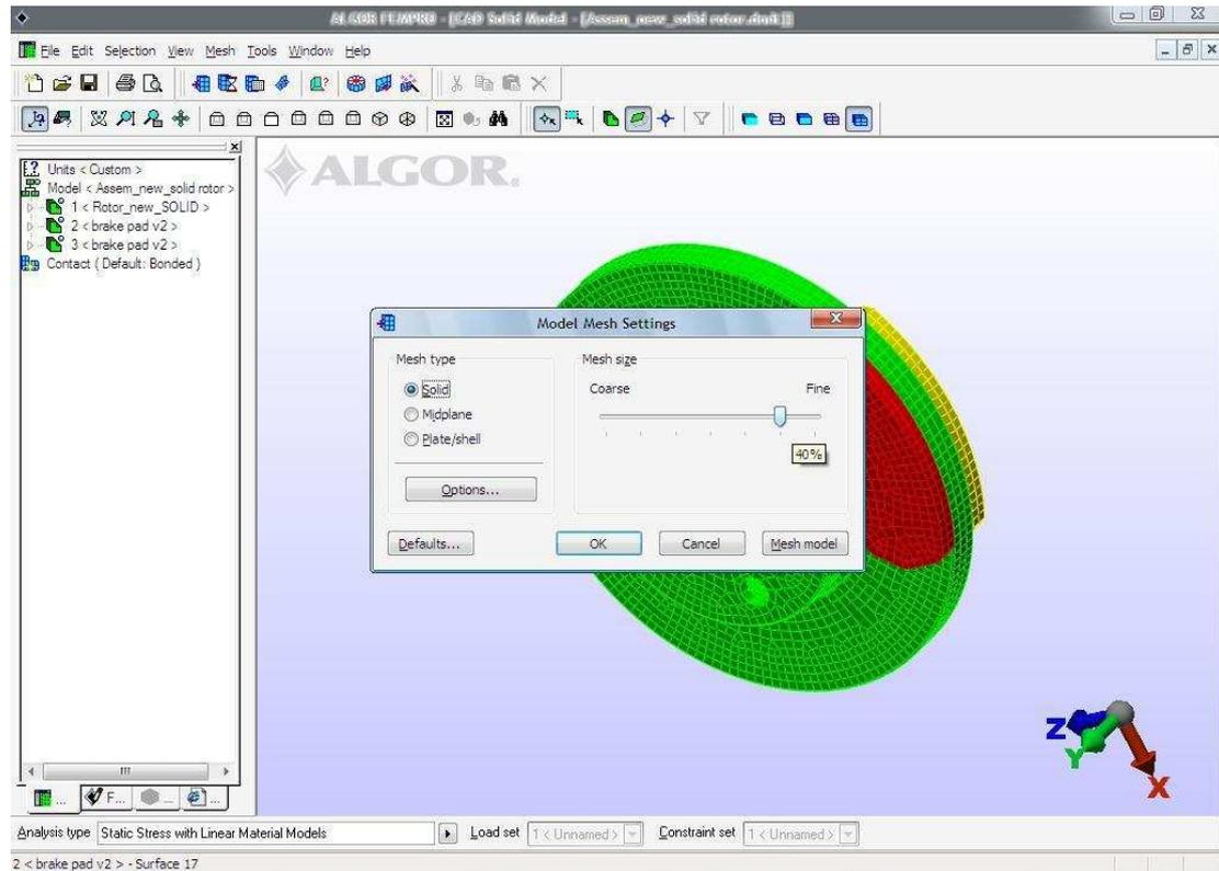
**Figure 3.6:** Model mesh size is set to 40%
