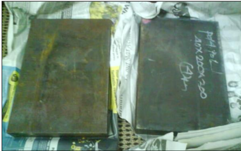
Figure 3.10: Raw material for mould (Mild Steel)
