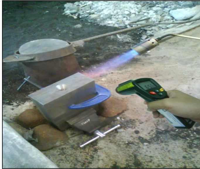
Figure 3.27: Temperature measure using Infrared Thermometer
