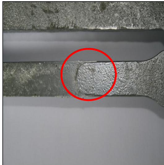
Figure 4.19: Cold shut at the tensile specimen
