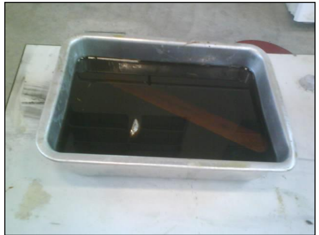
Figure 3.32: Cooling media using oil
