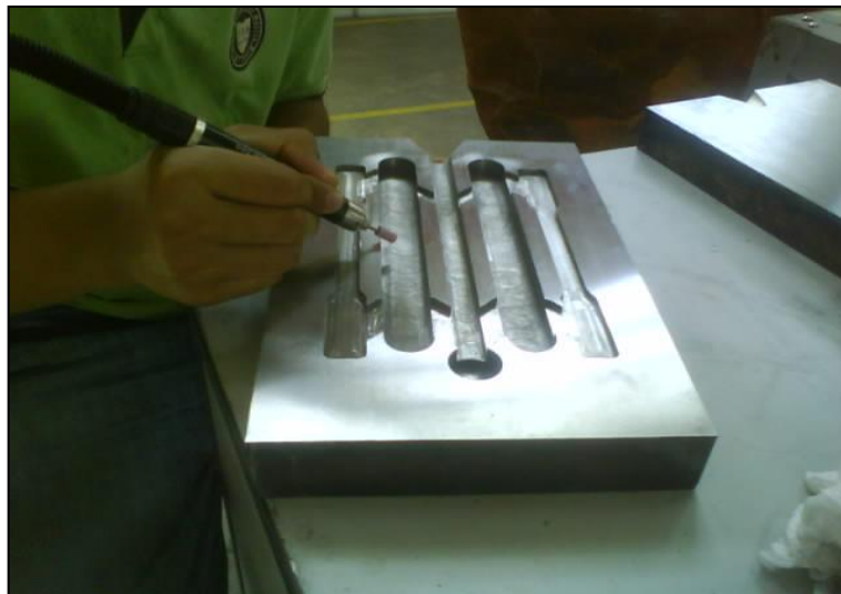
Figure 4.4: Finishing process using air grinder
