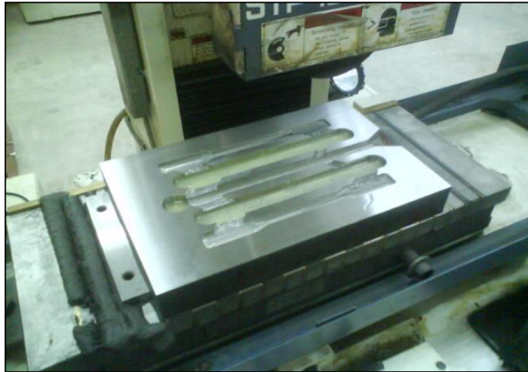
Figure 4.3: Finishing process using surface grinding machine
