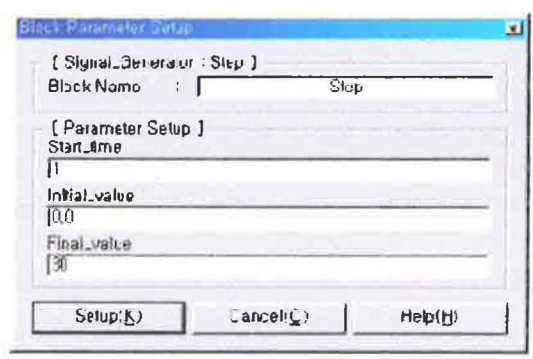
[Figure 5.8] Step Input Setup
