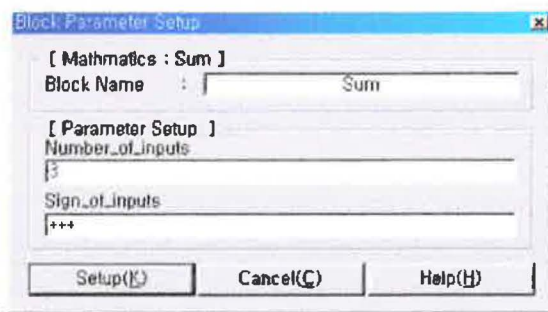
[Figure 2.21] Setup of Sum Block Parameter
