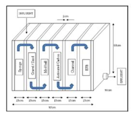
Figure 4: Illustration of mechanism of biofilter system
