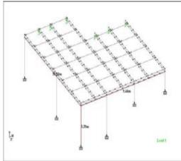
Figure 1. Car Porch Analyses using STAAD Pro 2007
