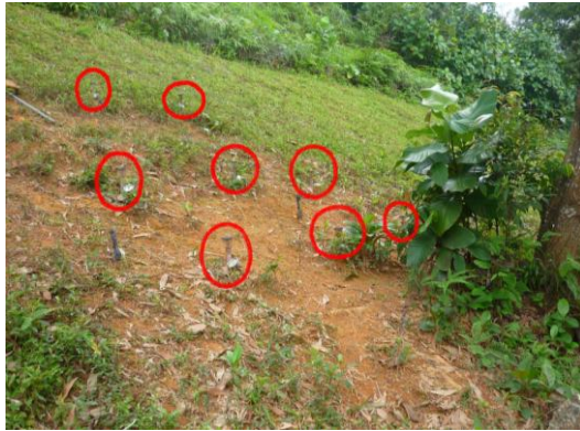
Figure 3 Tensiometer installed at slope
