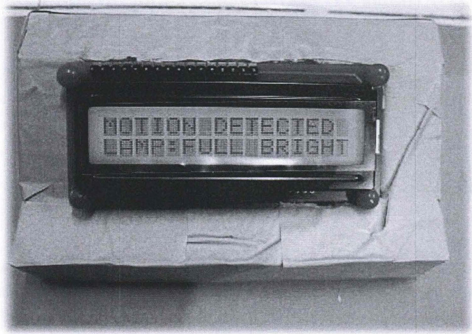
Figure 6.6: LCD screen display when LDR sensor sense intensity of light less than 0.4V and a motion has been detected
