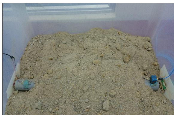
Figure 2(b). Buried pipe specimen
