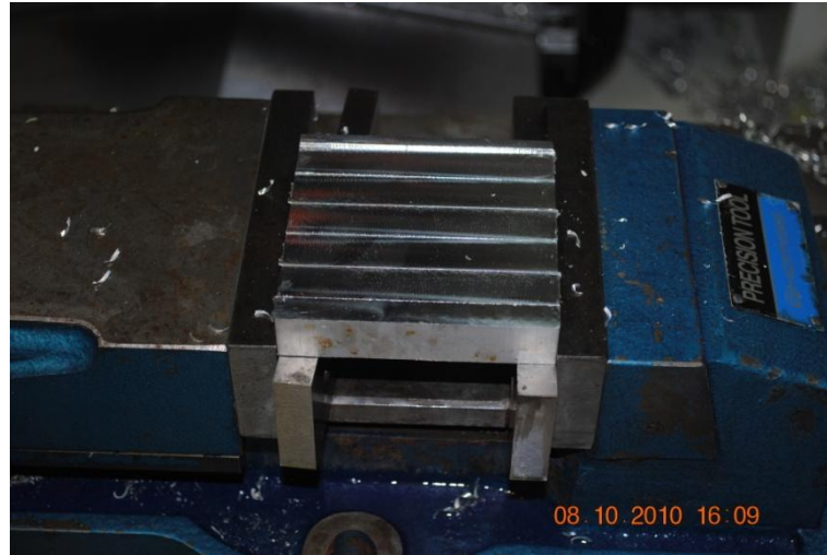
Figure 3.6 Aluminum Alloy T-6061 workpiece on the clamping devise
