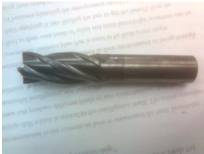
Figure 3.2 Flat endmill Tool with 4 flutes
