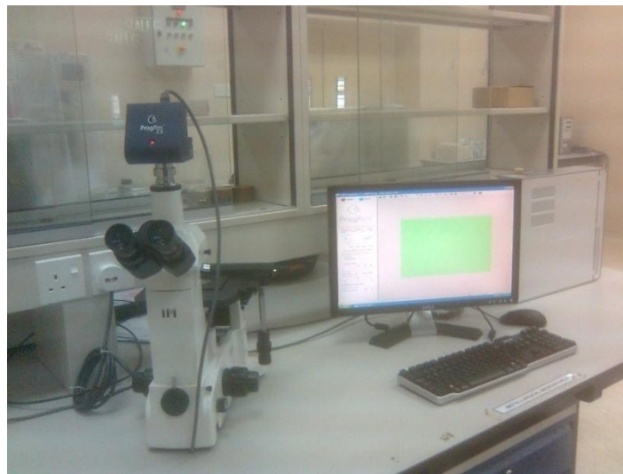
Figure 3.8 IM1700 Inverted Metallograph microscopes in FKM material Lab
