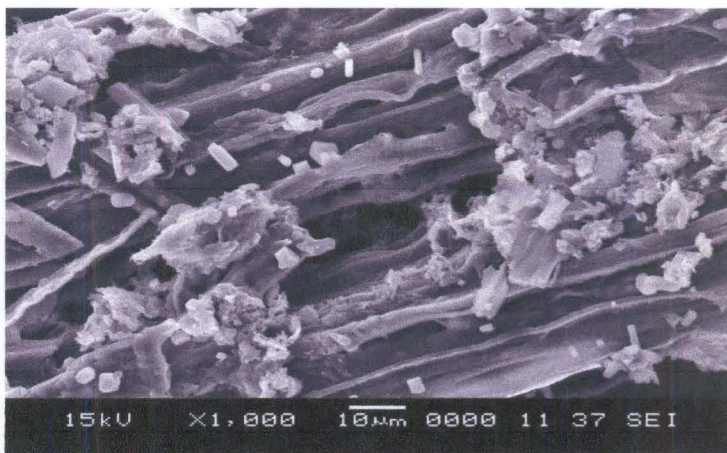
Fig 4: Surface morphology of Kenaf Fiber after HTC process at 6 h with stirring.
