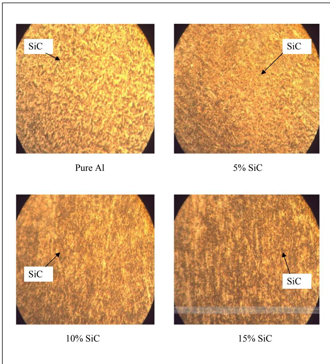
**Figure 4.6:** Microstructure for variation of wt% of SiC for magnification of 50X
