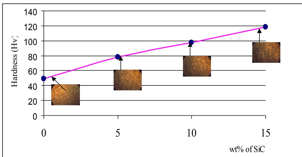
**Figure 4.1:** Graph of Vickers hardness against weight percentage of SiC
