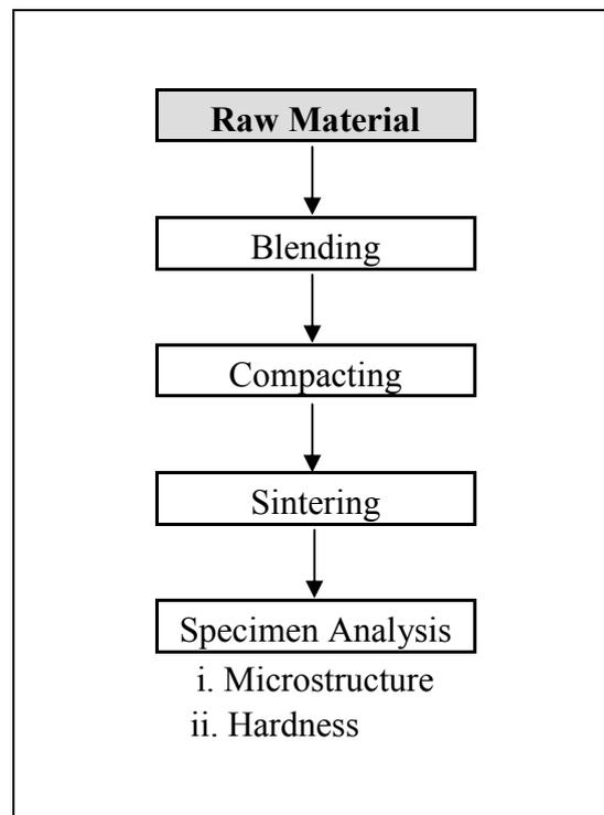
**Figure 1.1:** A flow chart of powder metallurgy method and specimen analysis
