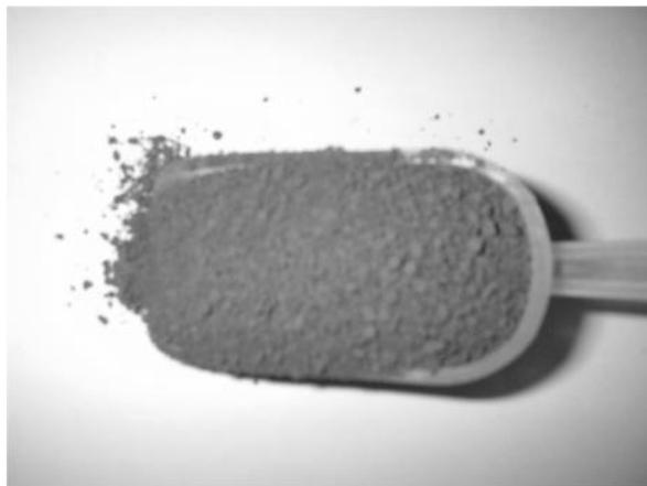
**Figure 3.8:** The resin used in hot mounting
