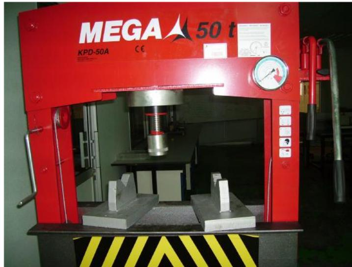
**Figure 6.5:** Hydraulic Power Pressure
