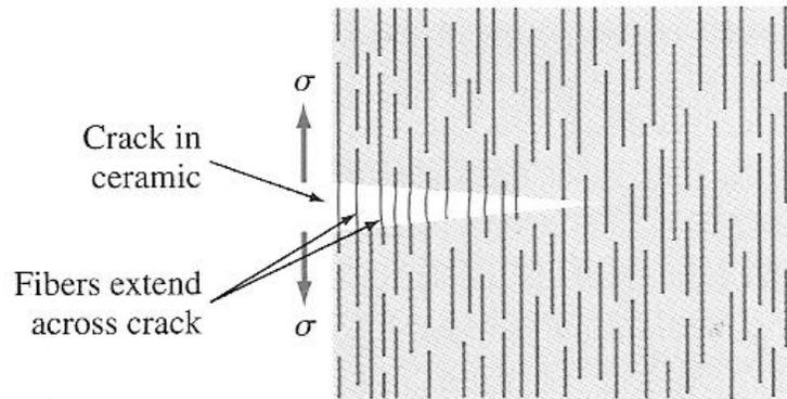
**Figure 2.2:** Schematic diagram showing how reinforcing fibers can inhibit crack propagation in ceramic matrix materials by crack bridging and fiber pullout energy absorption.
