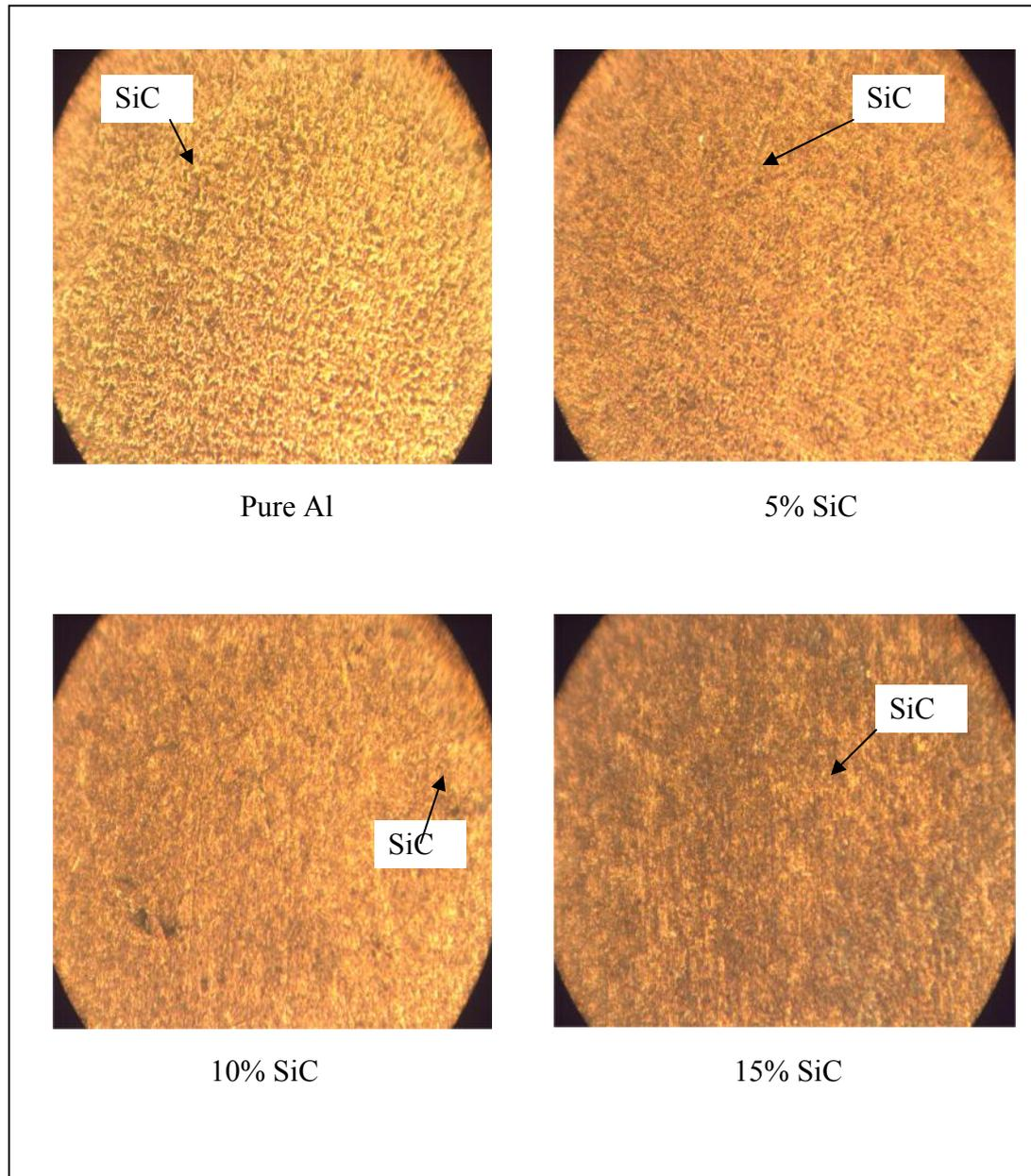
**Figure 4.5:** Microstructure for variation of wt% of SiC for magnification of 20X
