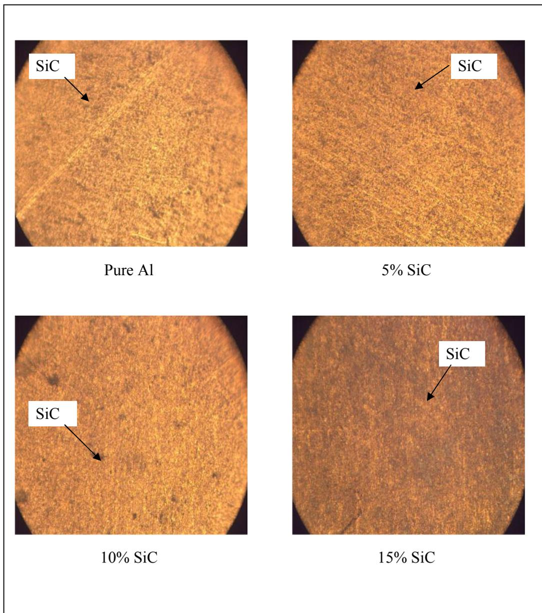
**Figure 4.4:** Microstructure for variation of wt% of SiC for magnification of 10X
