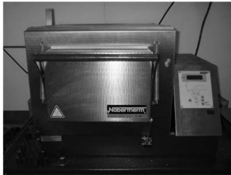
**Figure 3.6:** Heat Treatment Furnace that used in the sintering process
