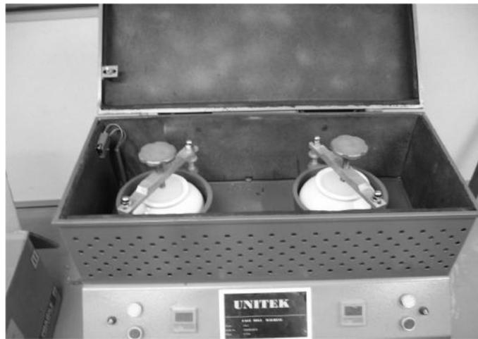
**Figure 3.4:** Fast Mill Machine that used to blend the composite
