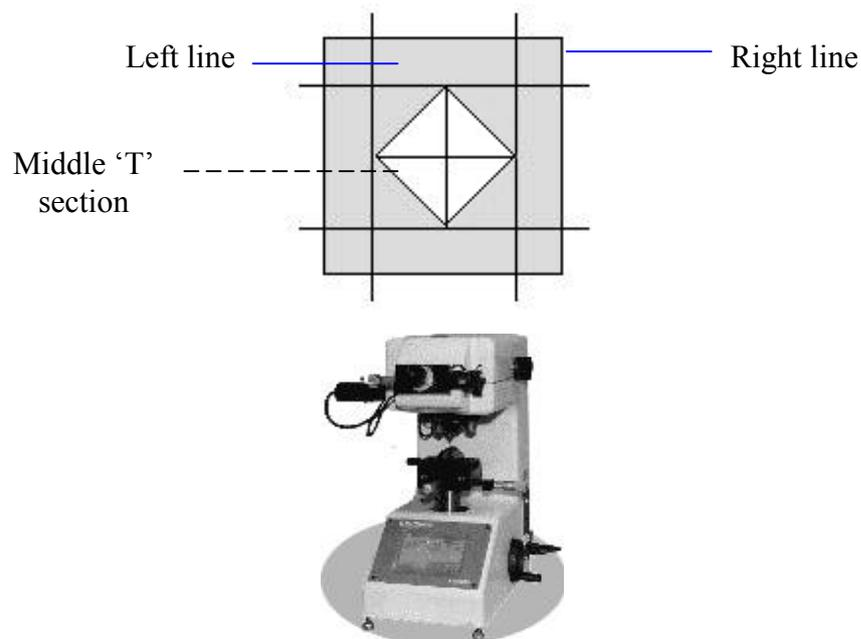
**Figure 3.11:** Digital micro hardness tester MMT-X7 Model
