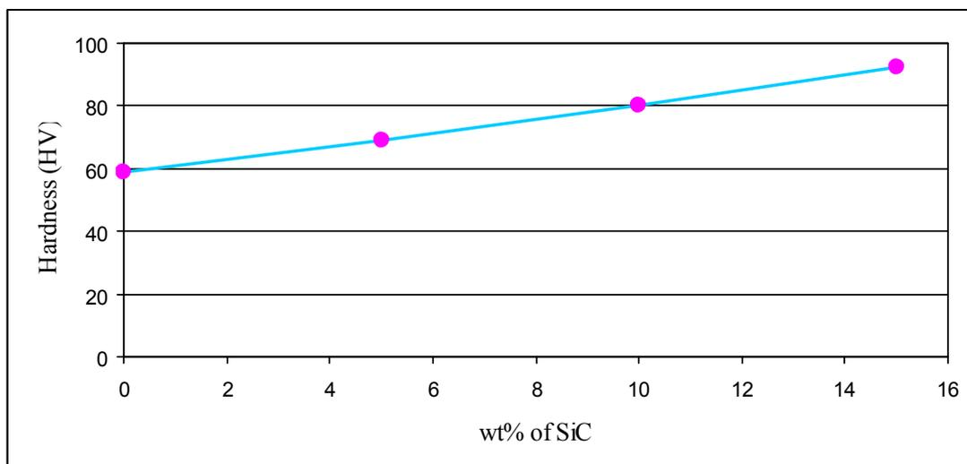
**Figure 4.2:** Graph of Vickers hardness against weight percentage of SiC based on the data from previous research
