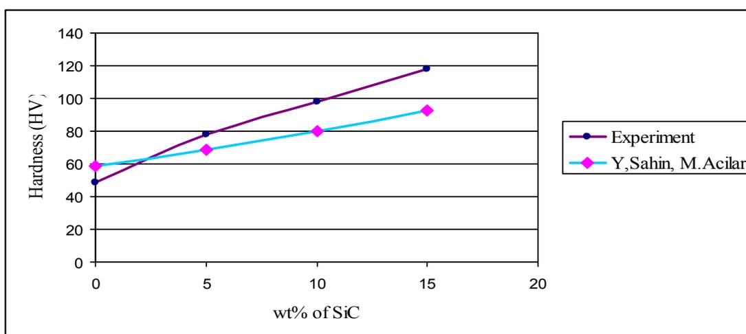
**Figure 4.3:** Comparison of Vickers hardness values between experimental values and previous research value
