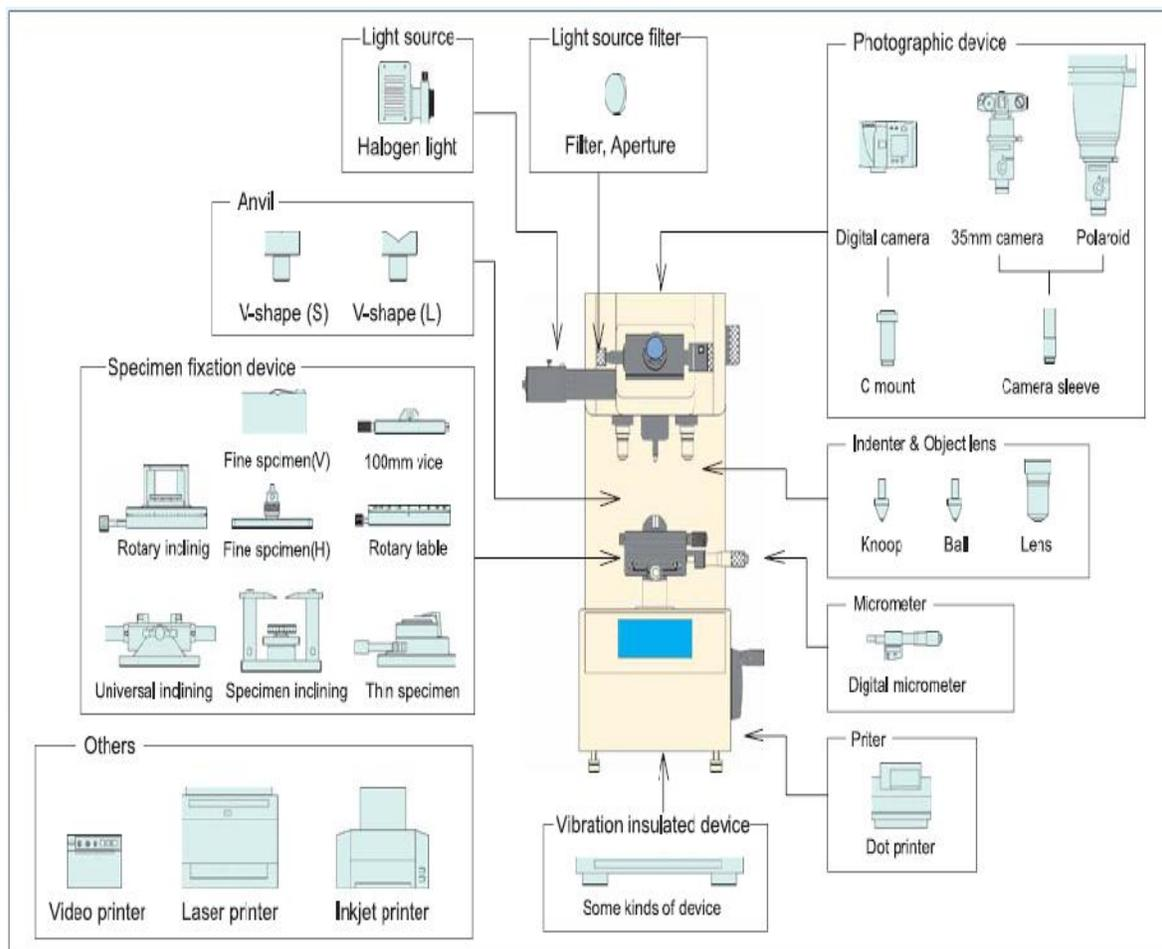
Figure 6.1: Vickers hardness tester
