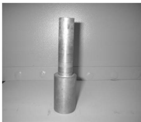
**Figure 3.2:** Experiment tools for powder compaction
