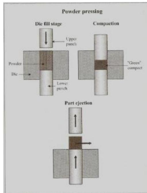
**Figure 3.5:** Powder compacting process
