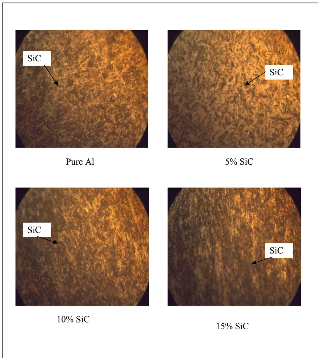
**Figure 4.7:** Microstructure for variation of wt% of SiC for magnification of 100X
