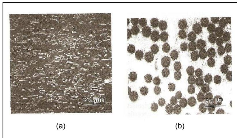
**Figure 2.1:** Typical microstructure of some metal matrix composites: (a) Particle (SiC particle/Al) and (b) continuous fiber reinforced (Al<sub>2</sub>O<sub>3</sub>/Al-Li) composites.
