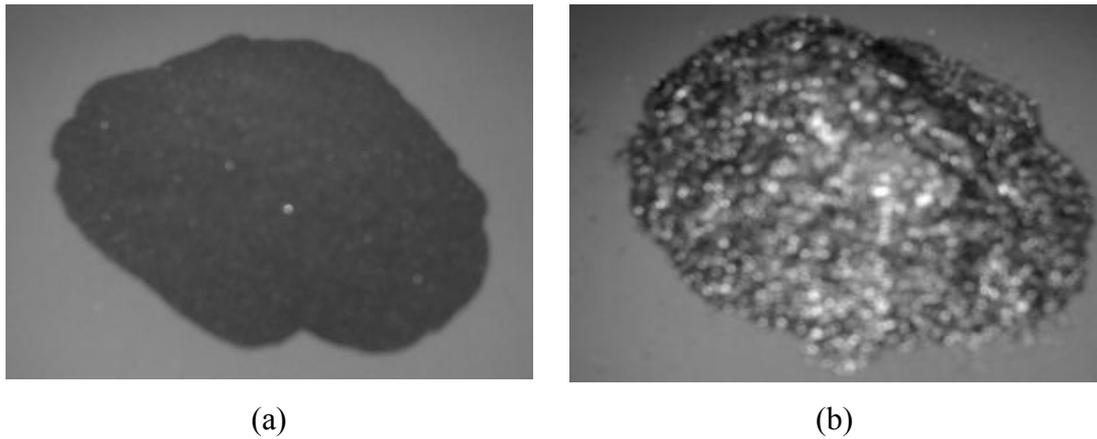
**Figure 3.3:** Raw material that used to produce composite. (a) Silicon carbide powder and (b) Aluminum powder
