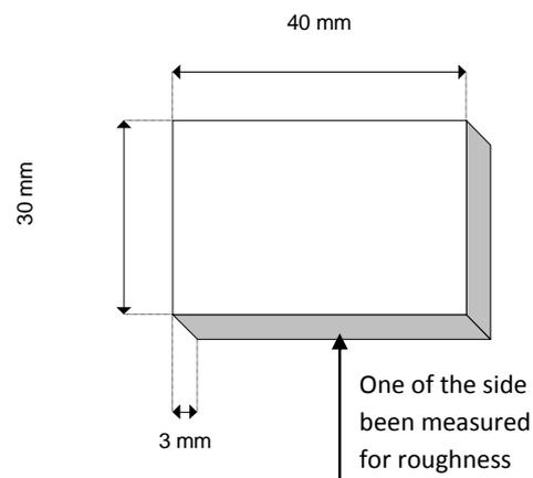
Figure 2: Dimension of the specimen
