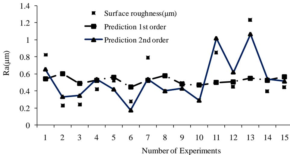
Figure 3: Comparison of RSM models against experimental values
