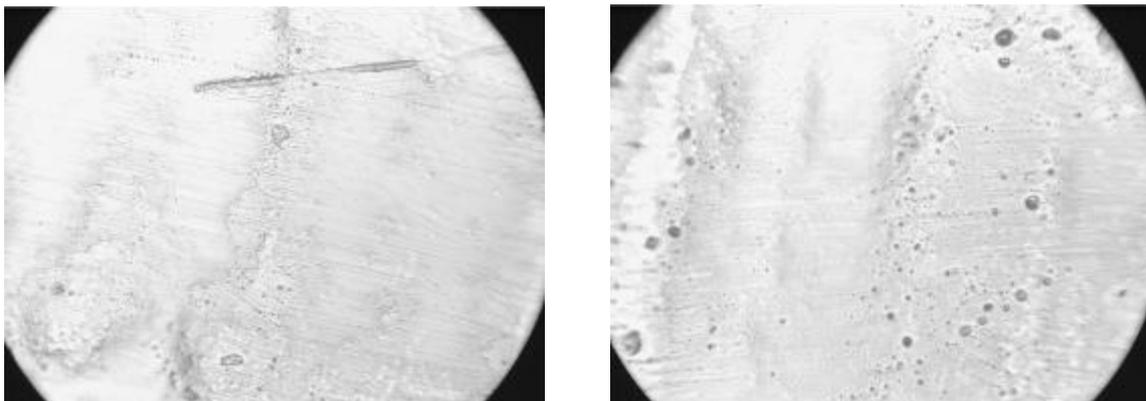
Figure 5: Microscope picture for roughness 0.277  $\mu\text{m}$
