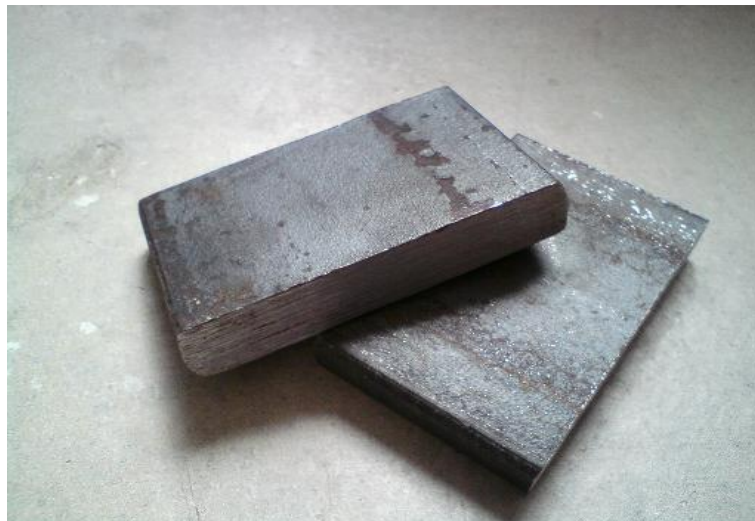
Figure E-1 : Raw material cutted by band saw machine
