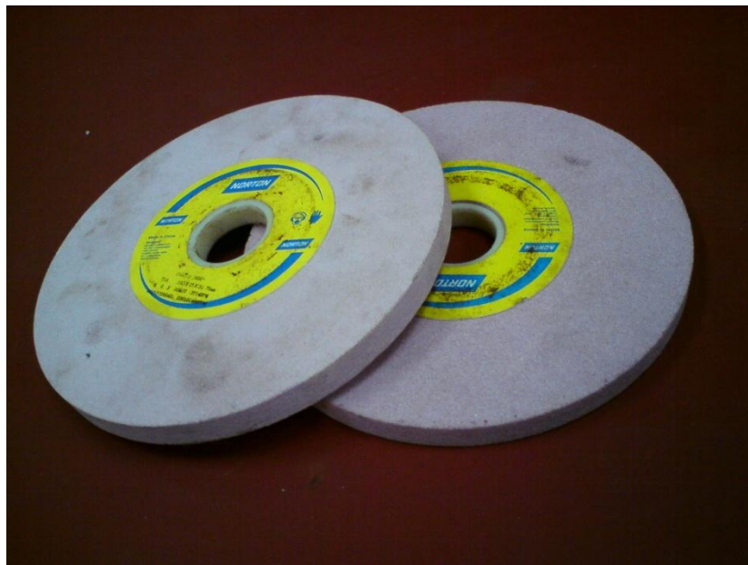
Figure 2.4 : Aluminium oxide wheel grinding
