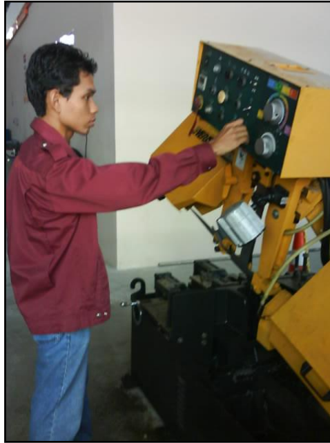
Figure B-1: Raw Material Cutting Process
