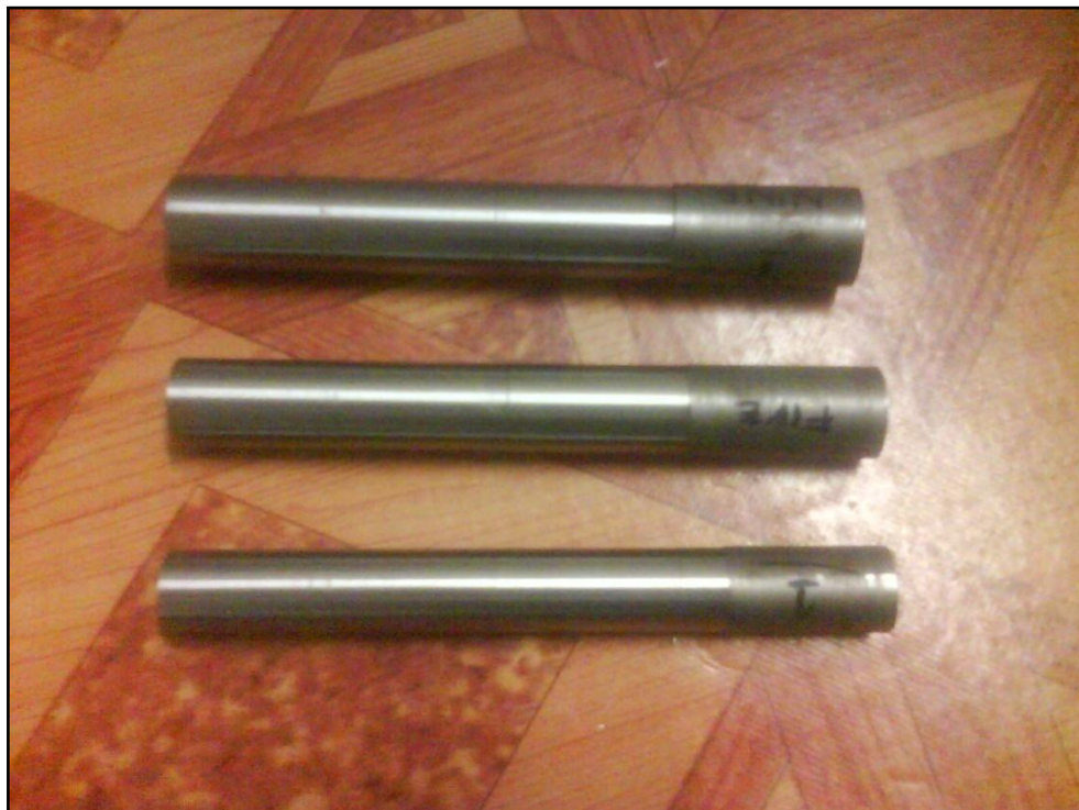
Figure 4.2: Three Work pieces After Grinding Process with Different Diameter
