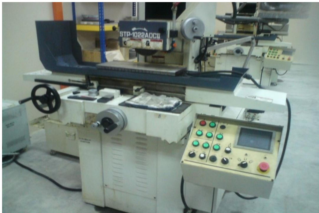
Figure 3.4: Transverse surface grinding
