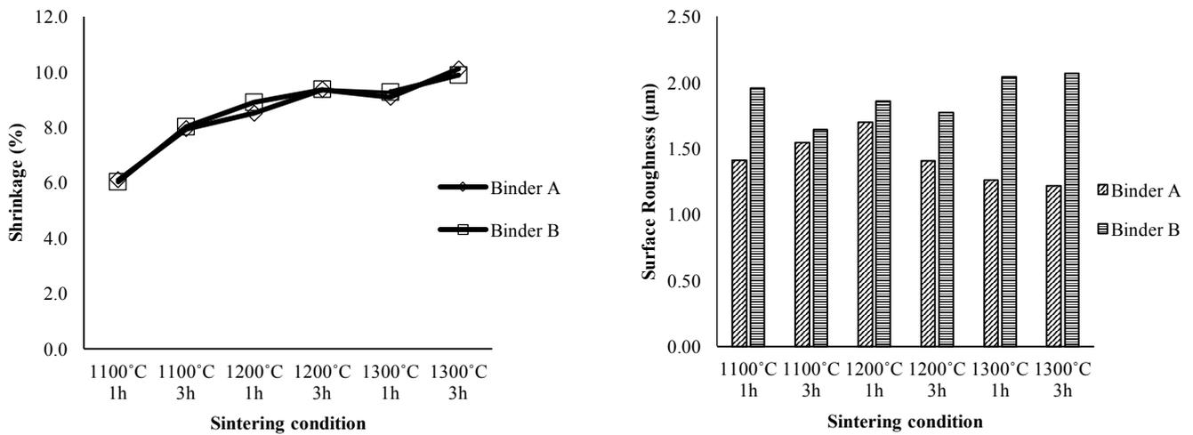
Figure 2: Dependence of shrinkage and surface roughness for binder A and binder B on MIM processing parameters
