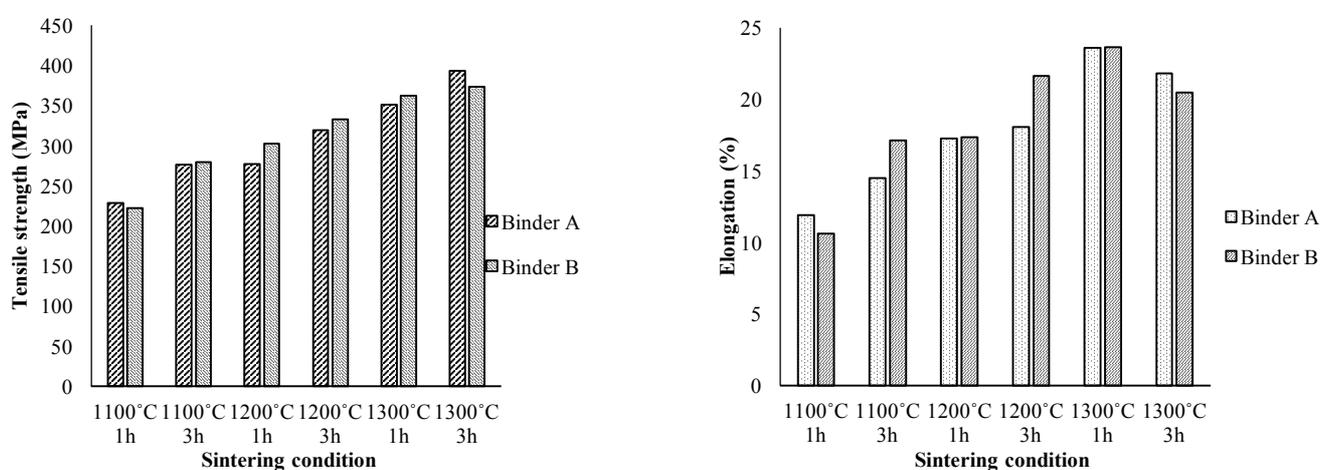
Figure 3: Tensile strength and elongation for binder A and binder B
