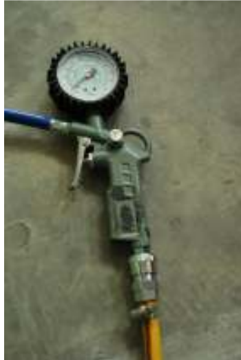
Figure 4.1: Pressure gauge use to measure the pressure
