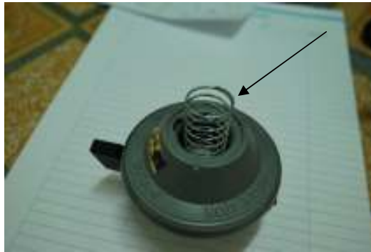
Figure 3.7: Pressure regulator spring that react to flow through it
