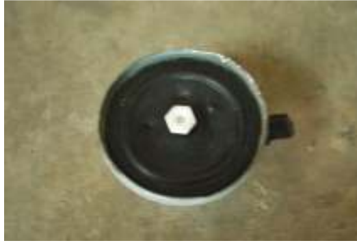
Figure 3.8: Pressure regulator diaphragm avoid any leakage of gas that flow through it
