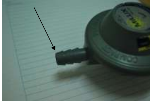
Figure 3.5: Pressure regulator outlet tube for gas outlet
