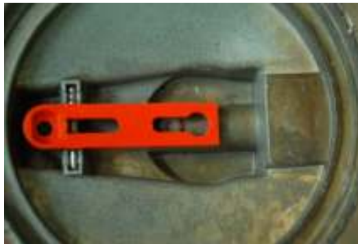
Figure 3.9: Pressure regulator caliper will react as the door for inlet tube
