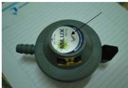
Figure 3.6: Pressure regulator top cover to protect the equipment in it
