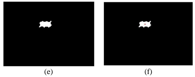
Figure 11 (a) Rectified Image captured from both Cameras (b) Mask the Target in the Captured Scene (c) Binary Image (d) Binary Image with Filled Holes (e) Segmented Image (f) COG of Segmented Image
