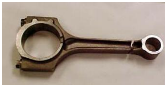
Figure 1.0: Failure of a connecting rod
