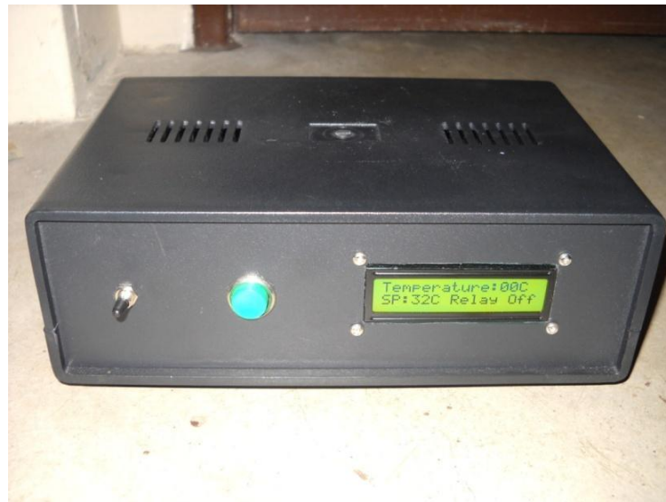
Figure 3.6: Heat management device
