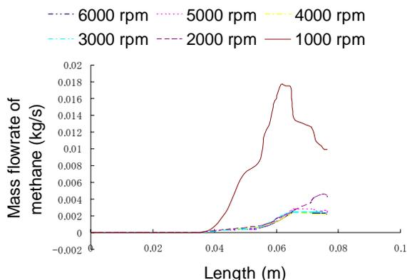
Figure 6: Methane mass fraction at different engine speed
