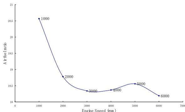
Figure 7: Air fuel ratio at different engine speed
