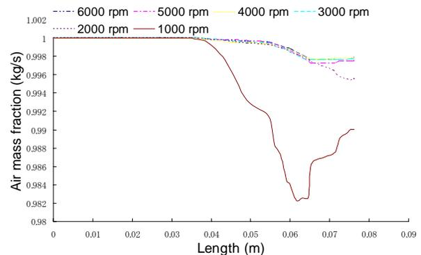
**Figure 5:** Air mass fraction at different engine speed
