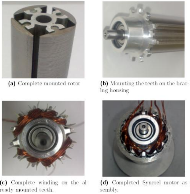
Fig. 3. The assembly of the Syncrel machine prototype.
