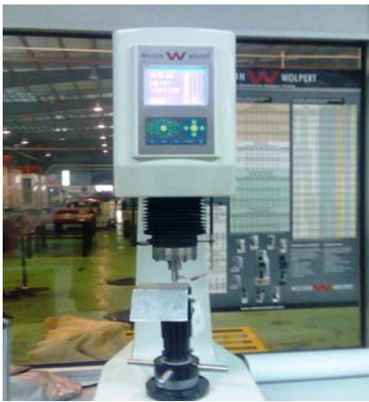
Figure 3: With digital display for Rockwell A, B, C and superficial hardness testing.
