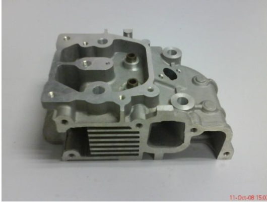
Figure 3.6 Actual Cylinder Head
