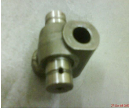
Figure 3.20 Actual connecting rocker arm
