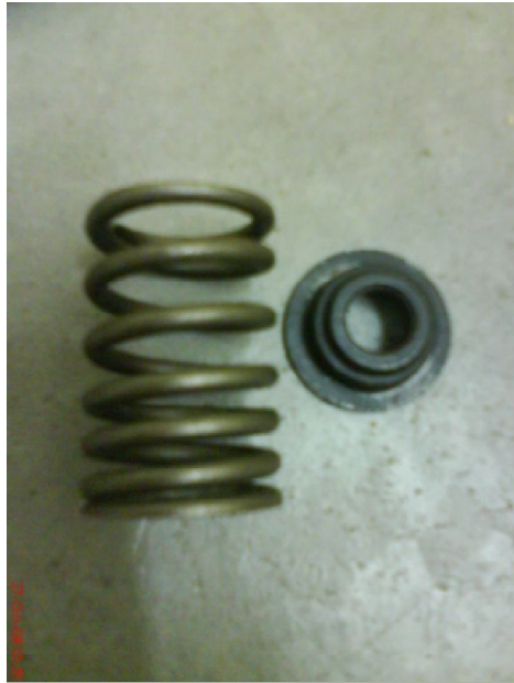
Figure 3.14 Actual spring and seat
