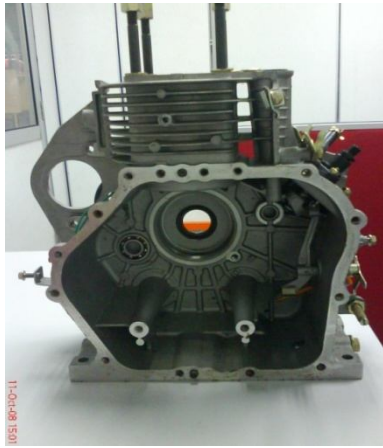
Figure 3.3 Actual cylinder blocks.
