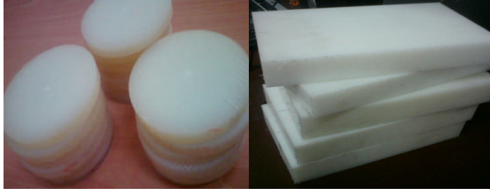
Figure 8: Nylon pieces that will be used to make the plates and the PE block for machining purpose
